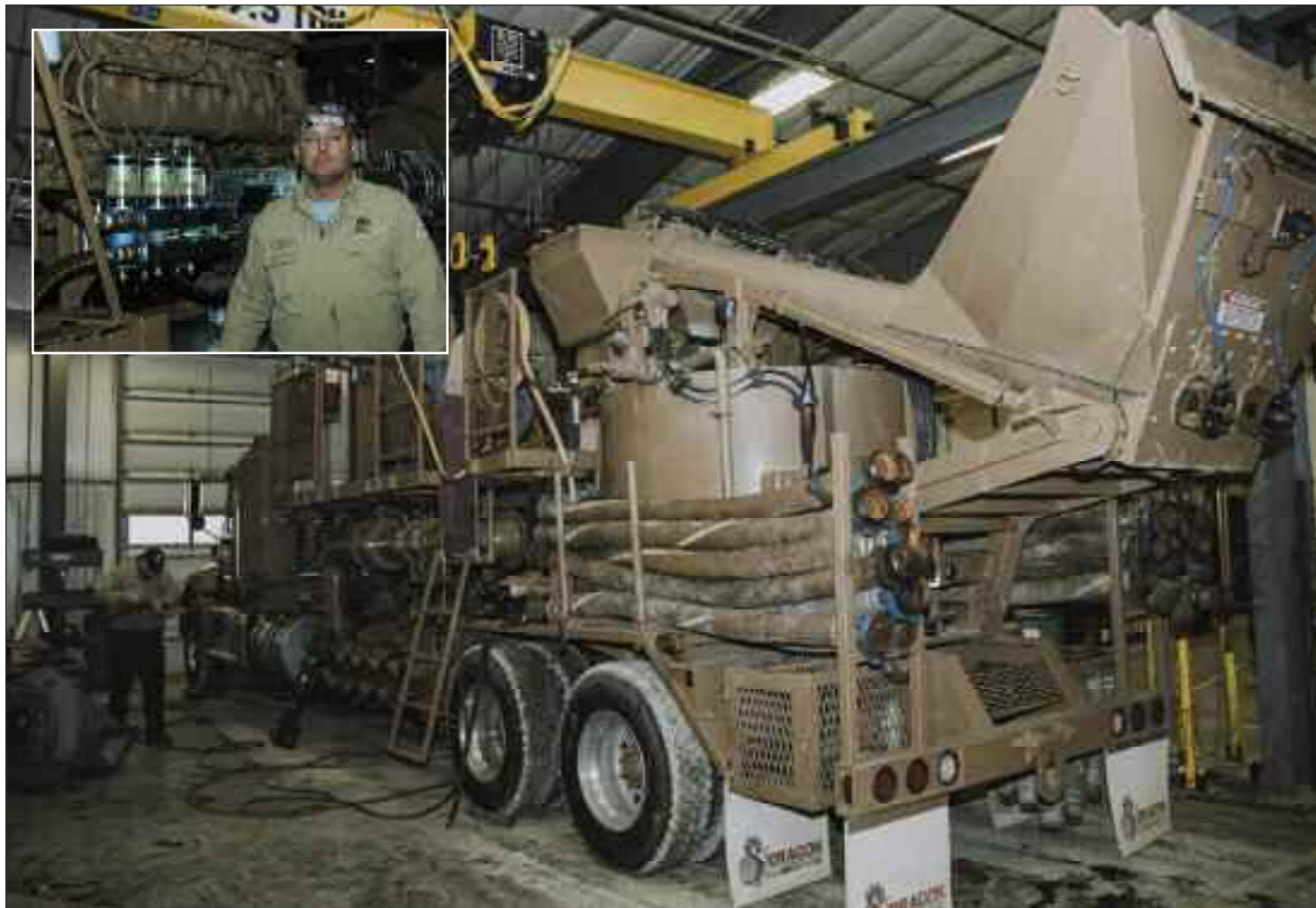
Maintenance technicians work on one of the company's blending units. The blender combines the sand, water and chemicals before sending it to the pump truck, which forces the mixture down the well at high pressures causing the shale to fracture. Inset: fabrication manager, Todd Lawler shows off a newly completed truck.
